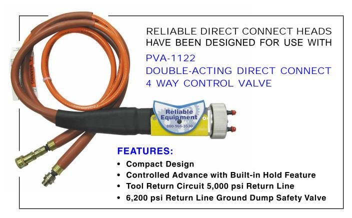
Open center 4-way, 3-position control valve used for controlling double-acting Crimping Heads and Cutters. Connect directly to the tool or use with high pressure hoses for remote operation. The Pivot Style Control Valve may be operated with one hand, leaving the second hand free to control the head.
