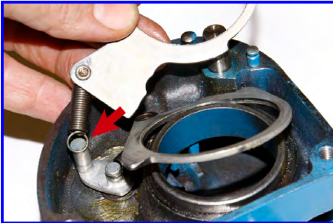
Remove Free Chain Ring and Spring from Control Mechanism.
