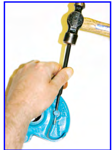
Drive Control Lever from Mechanism
