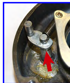
Remove Mechanism through Hoist Body.
