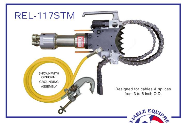
The REL-117SM double acting hydraulic spearing tool was designed to drive a serrated piercing blade into the conductor or joint ensuring that the conductor is out of service prior to beginning work.
