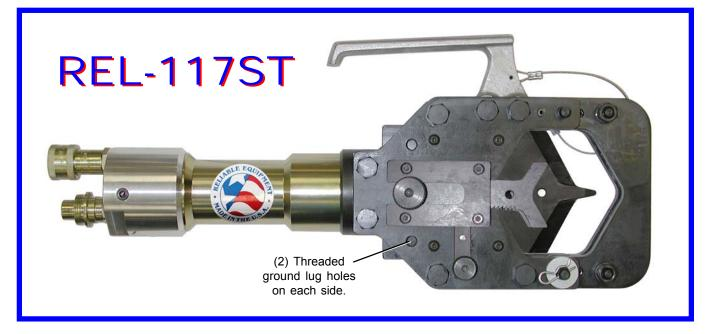
The REL-117 double acting hydraulic spearing tool was designed to drive a piercing blade into the conductor, ensuring that the conductor is out of service, prior to beginning work.
