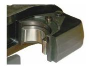
Ensure that you are using the proper die, as recommended by the connector manufacturer.
