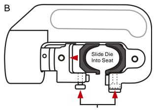
Tighten Thumb Screws to Secure Kearney Type Dies
