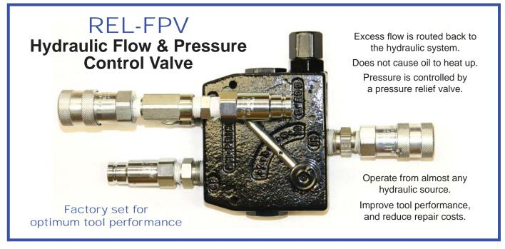
Hydraulic systems running in excess of acceptable tool pressure or flow may be corrected with the addition of an in-line pressure or flow reduction valve.
