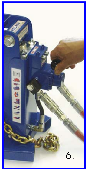
Move control valve in the DOWN direction and repeat process as required
