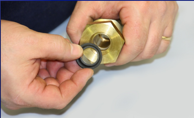
Install Ram Wiper At The Bottom Of The Packing Nut
