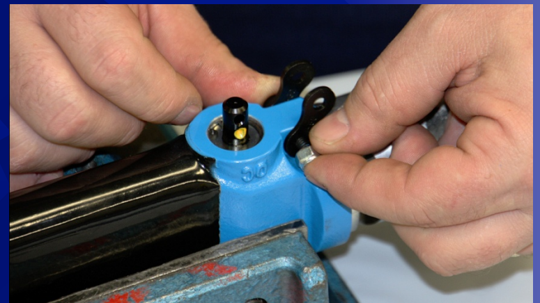
Install Locking Hex Nut
