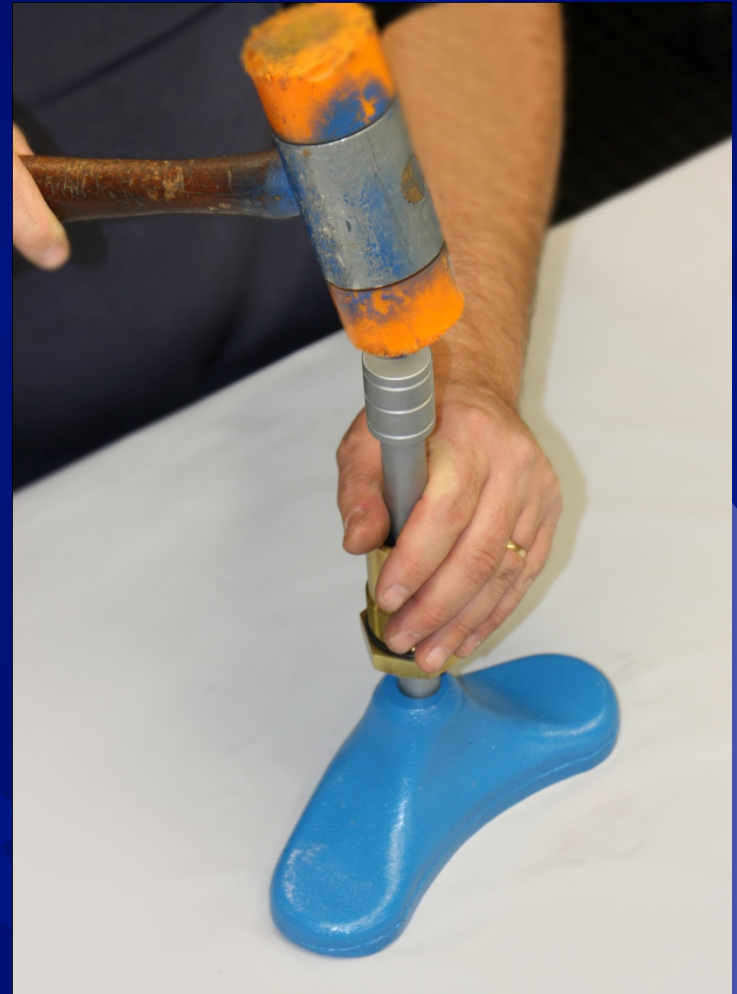
A Mallet May Be Used To Seat Ram Completely Into Assembly
