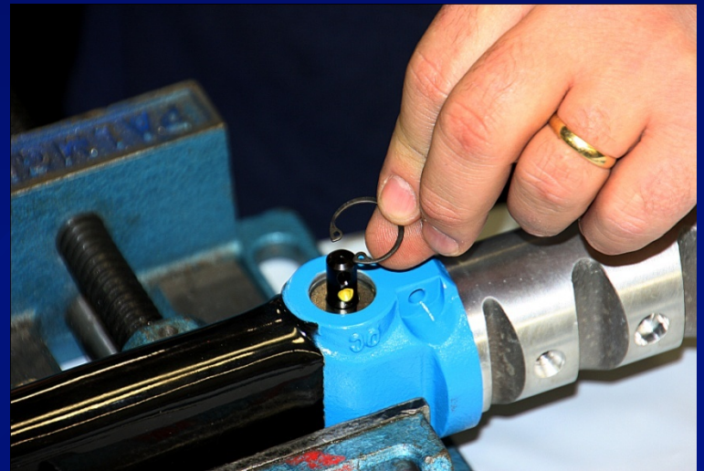
Insert Spring Clip Over Spool Washer
