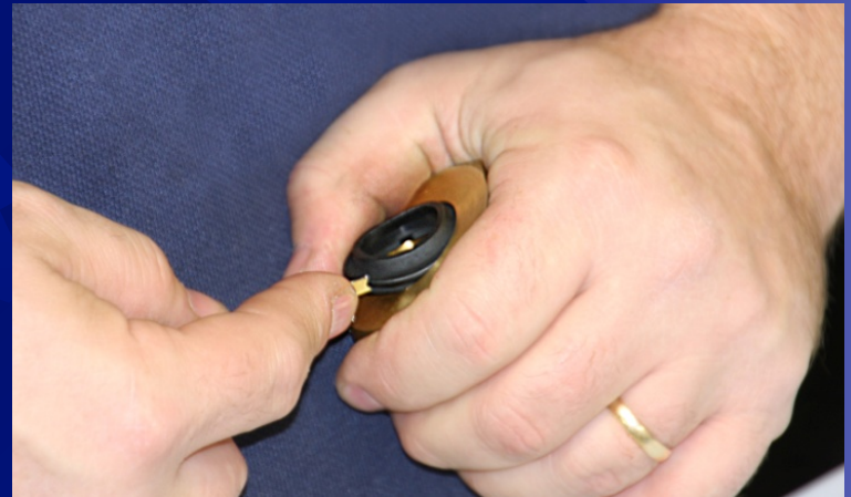
Install Ram Wiper At The Bottom Of The Packing Nut
