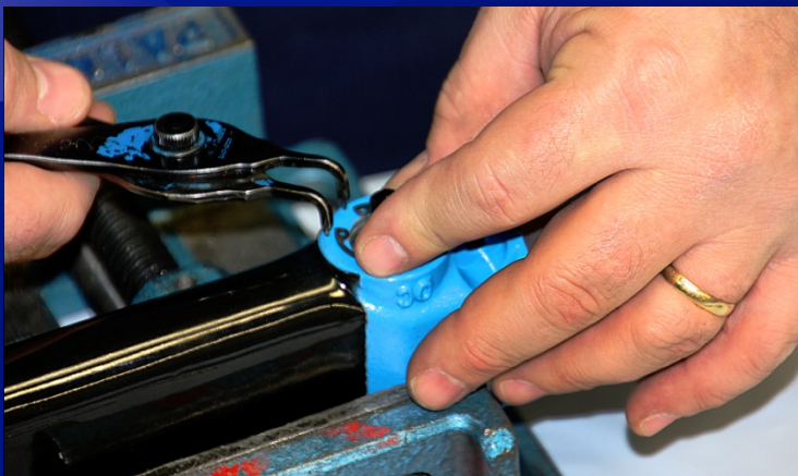
Work Clip Into Handle And Ensure That Clip Is Seated Securely
