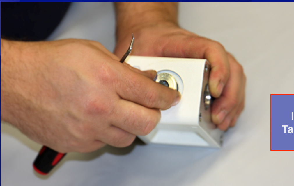
Install O-Ring Over Plug
