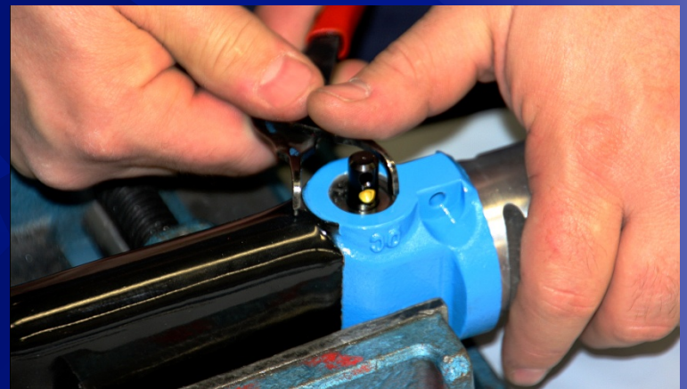
Work Clip Into Handle And Ensure That Clip Is Seated Securely
