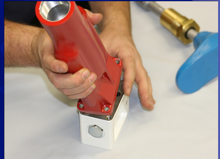
Seat Drive Shaft Completely And Install Body Onto Valve Body
