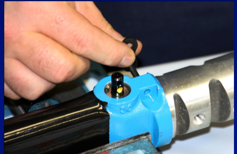
Insert Cap Screw Through Handle
