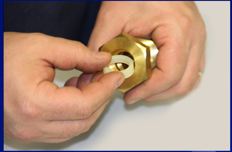
Install U-Cup Seal Into Inner Wall Of Packing Nut
