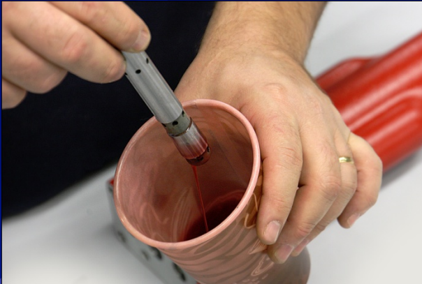
Lubricate Drive Shaft & Install Into Body
