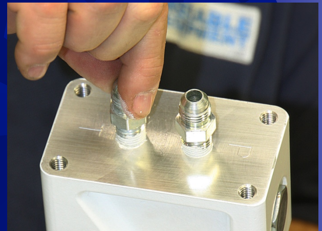
Apply Thread Sealant To Hydraulic Adapters
