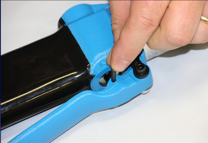
Insert Spring Pin Into Trigger
