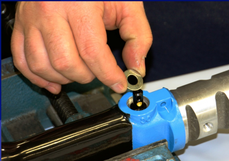
Insert Spool Washer Into Handle
