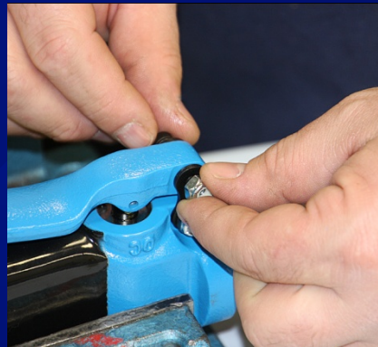
Install Locking Nut Onto Cap Screw
