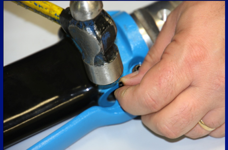
Drive Spring Pin Flush With Trigger
