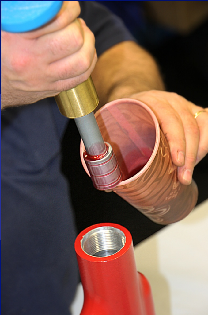
Lubricate Ram Assembly and Insert Into Tamper Body
