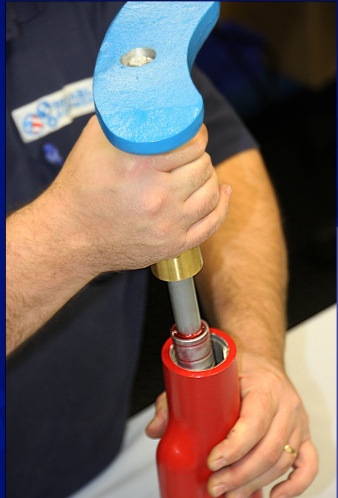
Lubricate Ram Assembly and Insert Into Tamper Body
