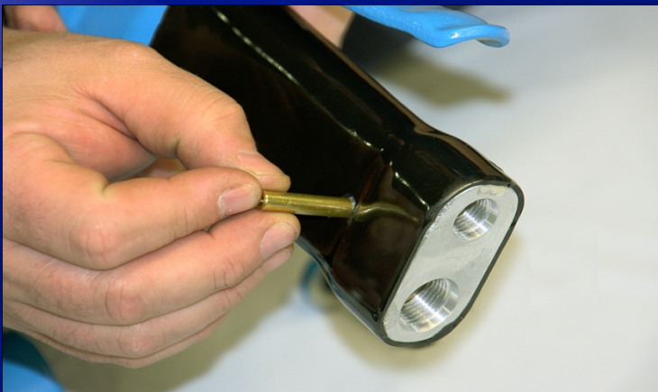
Insert Brass Sleeve Into Handle
