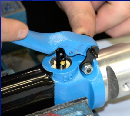
Install Locking Nut Onto Cap Screw
