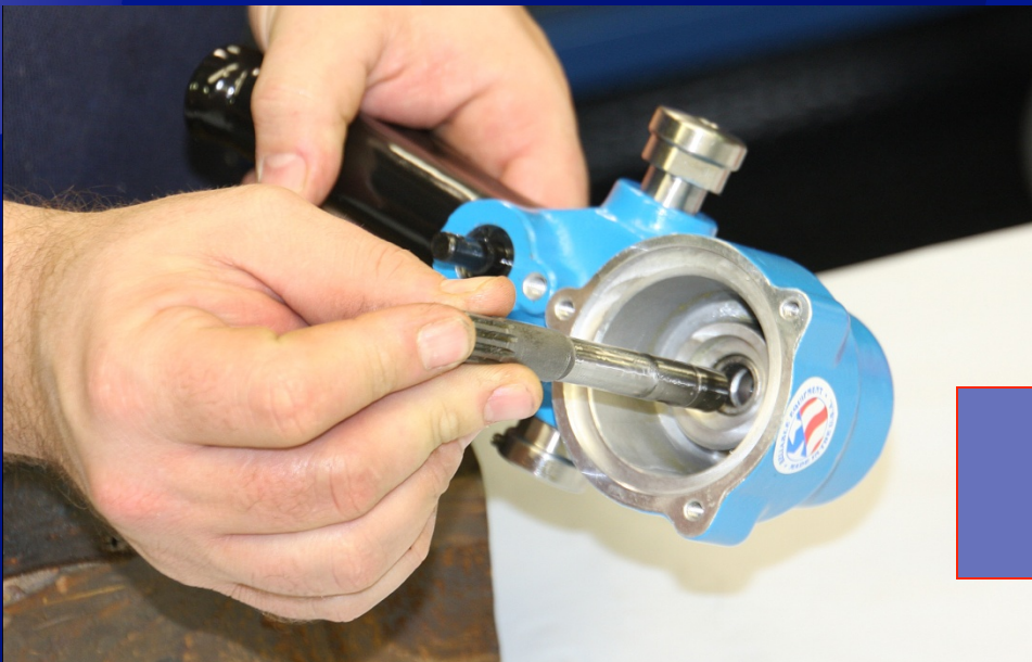
Insert Drive Shaft Through Tool Body
