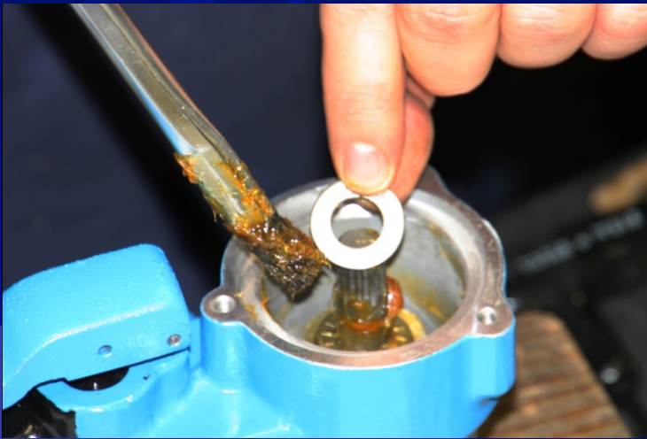
Install Washer & Apply Grease
