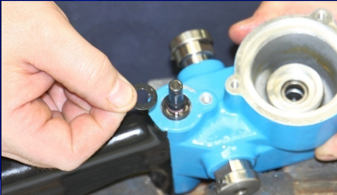
Slide Washer Onto Spool
