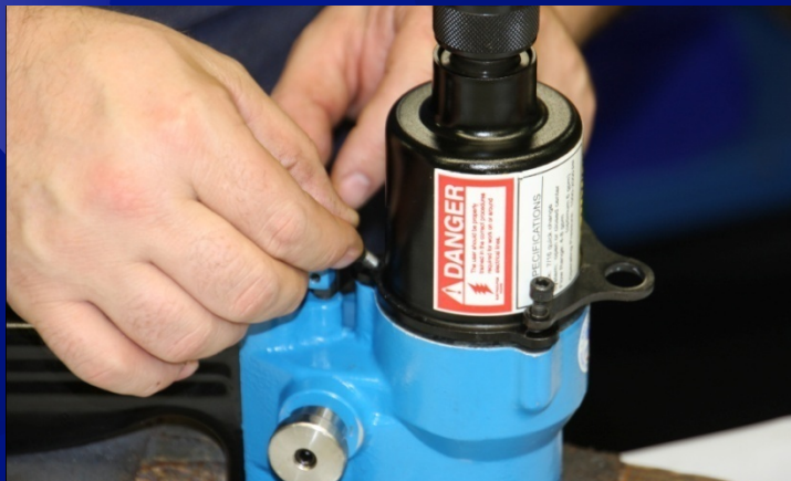
Install Nose & Hanger Assembly
