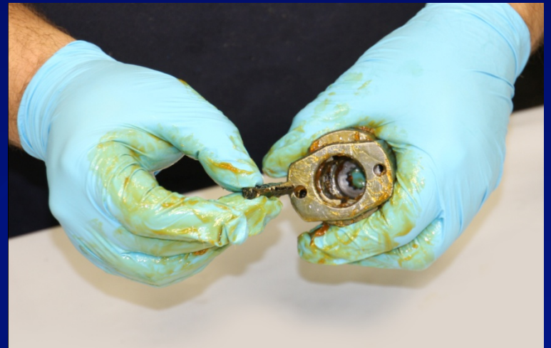
Align & Insert Hammer Pin
