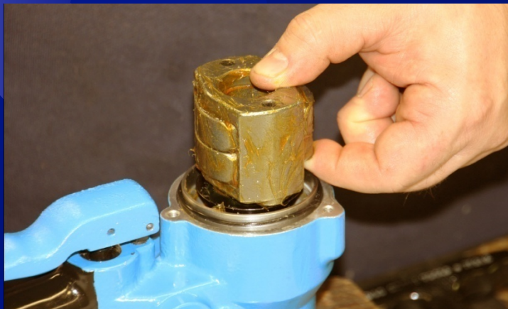
Cage Must Mesh With Drive Shaft
