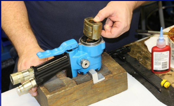
Place Cage Assembly Onto Tool
