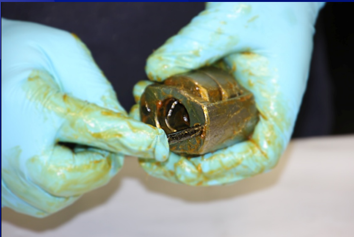
Install Second Hammer Pin
