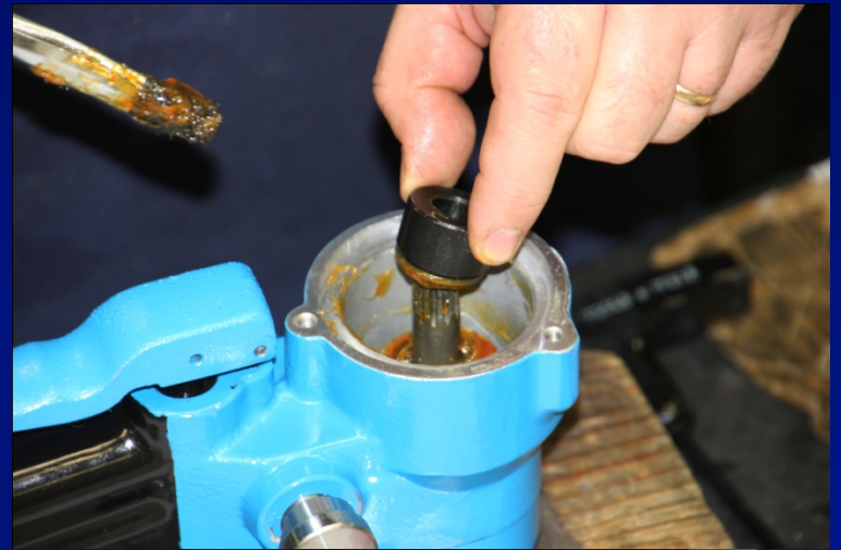
Install Spacer & Apply Grease
