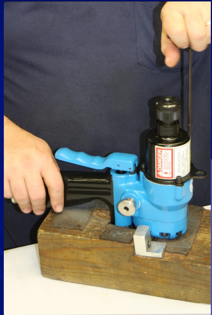
Tighten (3) Front End Screws
