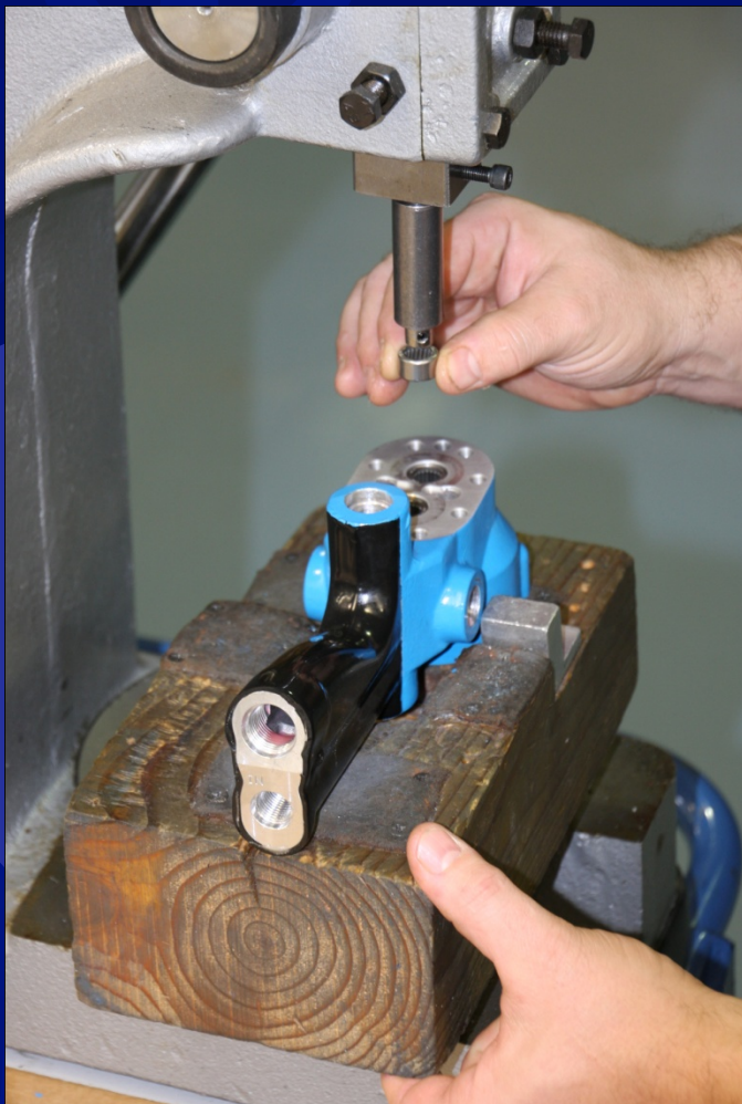
Press Upper Bearing Into Tool Body
