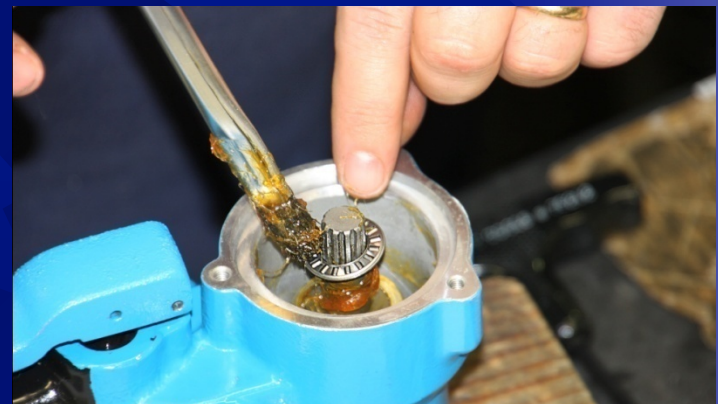
Install Thrust Bearing & Grease
