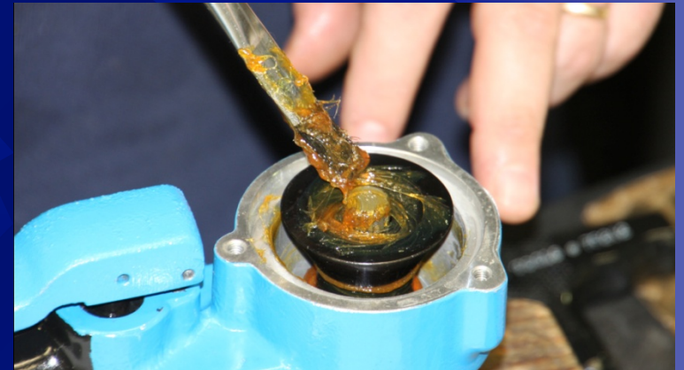
Apply A Coating Of Grease
