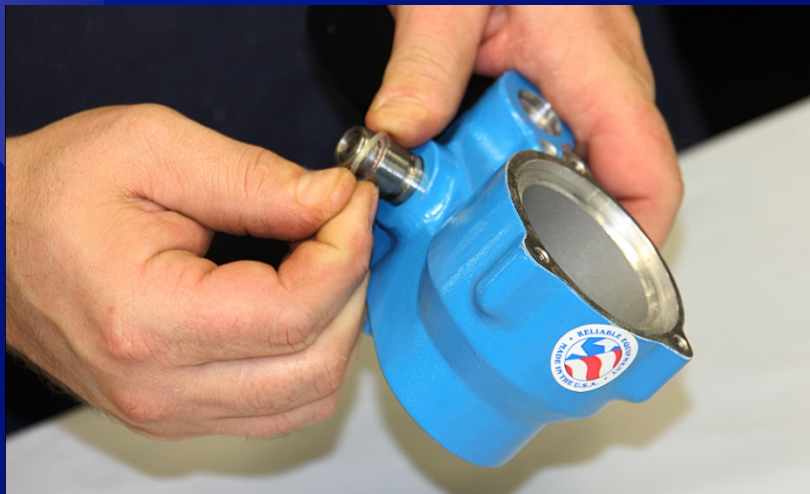
Install O-Ring To First Groove Of Spool
