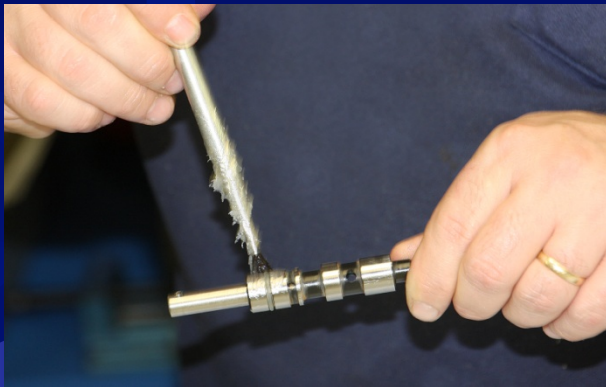
Lubricate Spool Assembly
