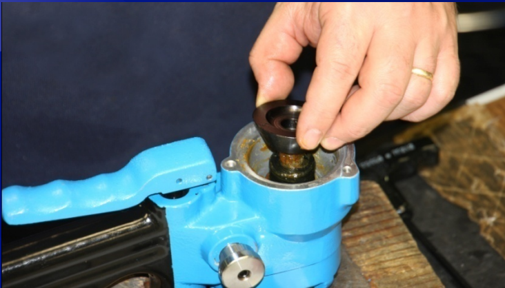
Install Pin Washer
