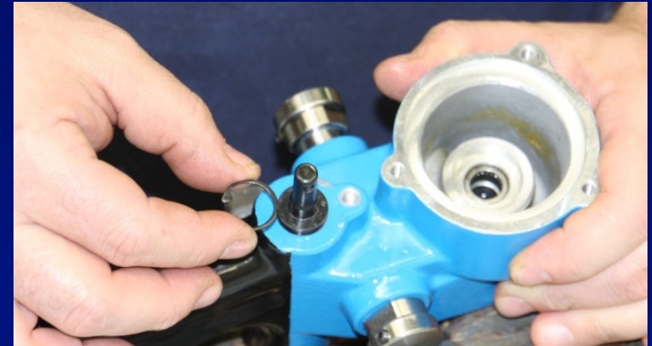
Install Snap Ring To Secure Spool
