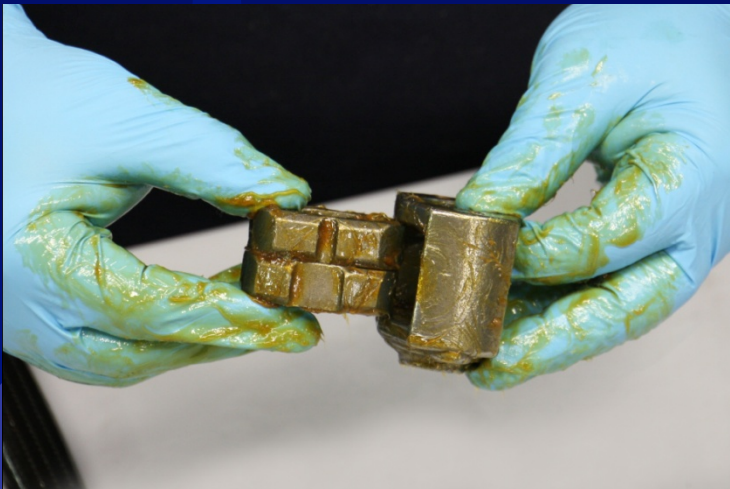
Assemble Hammers Into Cage
