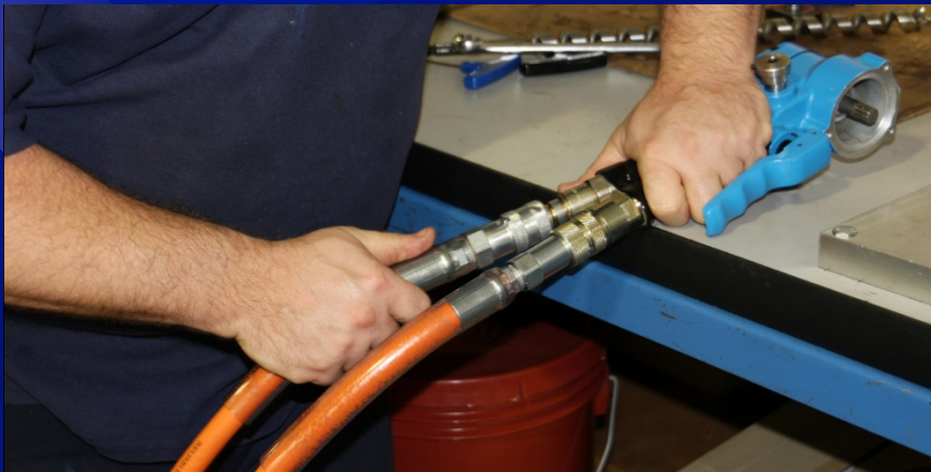
Connect To Hydraulic Test Source
