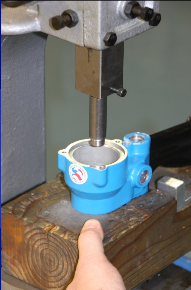
Press Inner Bearing Into Tool Body
