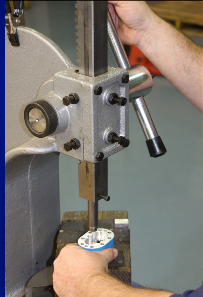
Press (2) Bearings Into Motor Cap
