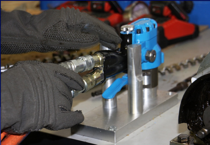
Mount Into REL-425TS Test Stand
