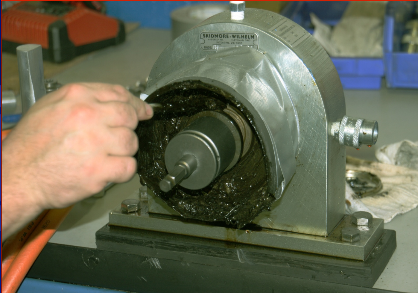
Apply Lubricant To Skidmore Test Machine
