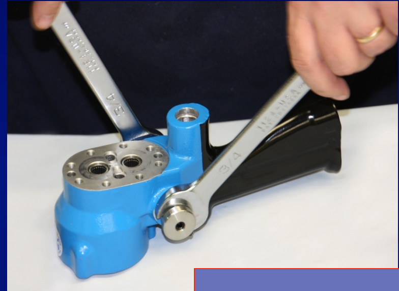
Use Two \frac{3}{4} Inch Open End Wrenches To Tighten Caps
