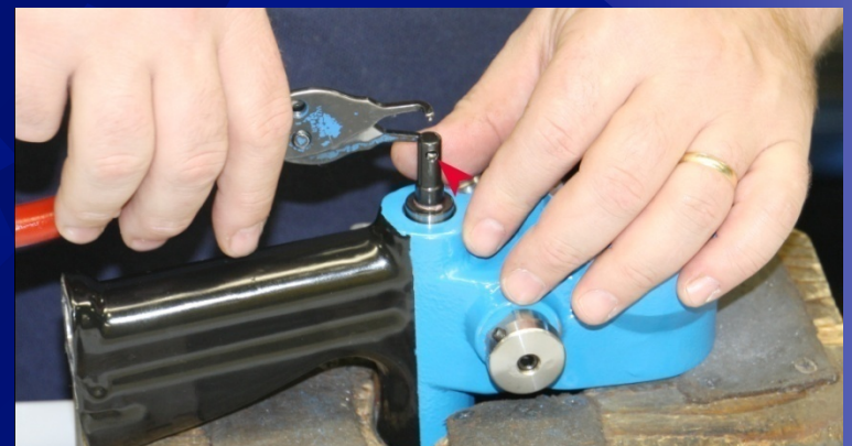
Align Spool For Trigger Installation
