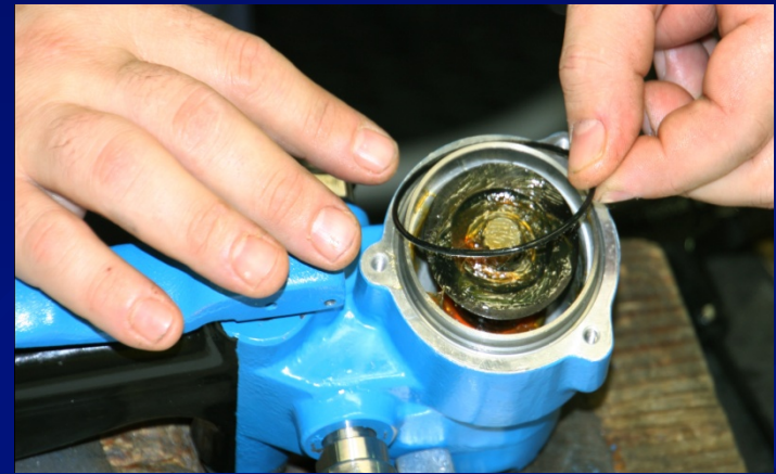
Install O-Ring Over Flange
