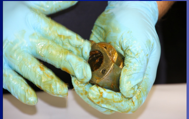
Re-Apply Grease To Assembly
