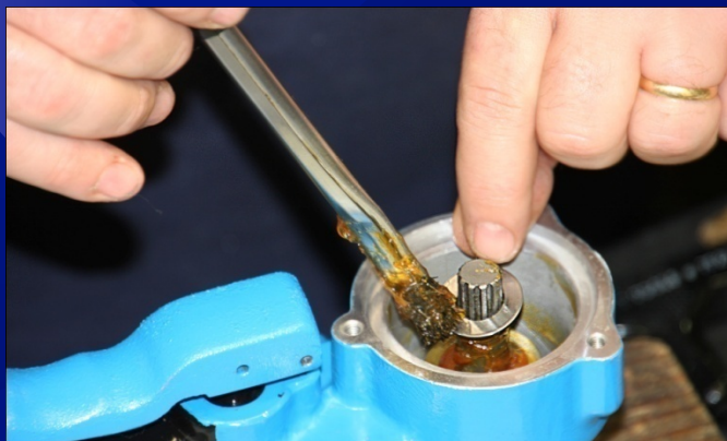
Install Washer & Apply Grease
