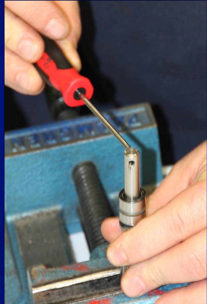
Back Stem Out To Clip This Is Open Center Setting
