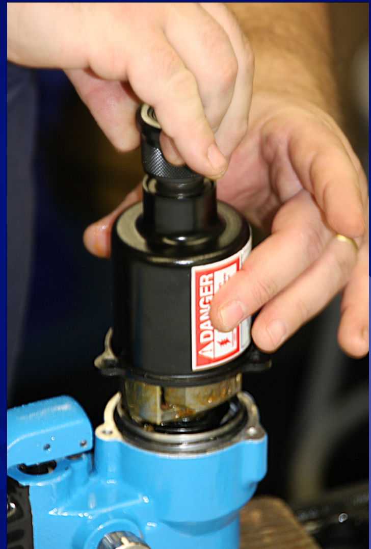
Install & Align Nose Assembly
