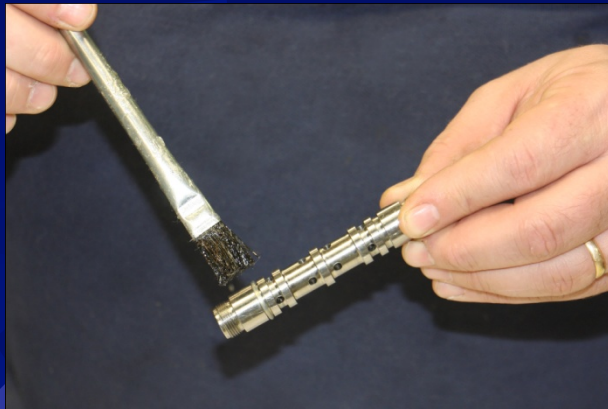
Lubricate Spool & Install Into Impact Body
