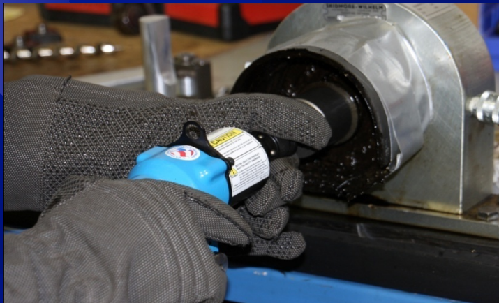
Test Torque On Skidmore Unit
