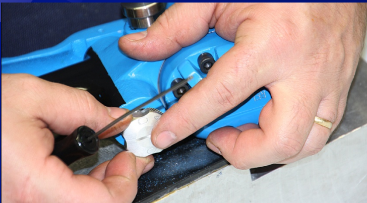
Install OC Knob Onto Spool
