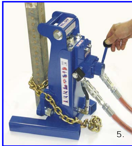
Move control valve into the UP direction to begin lifting post.
