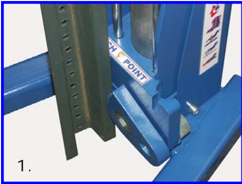
Slide flanged post between jaws.
