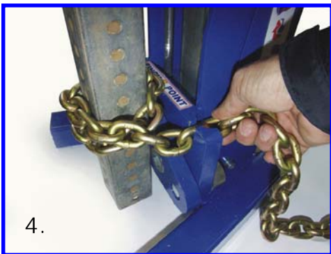
Insert chain section securely into second connection point as shown.
