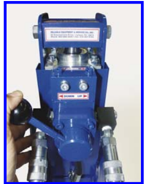
Move control valve into DOWN direction before inserting post or chain.
