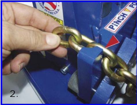
For square and solid posts place base around post and insert chain end into connection point as shown.
